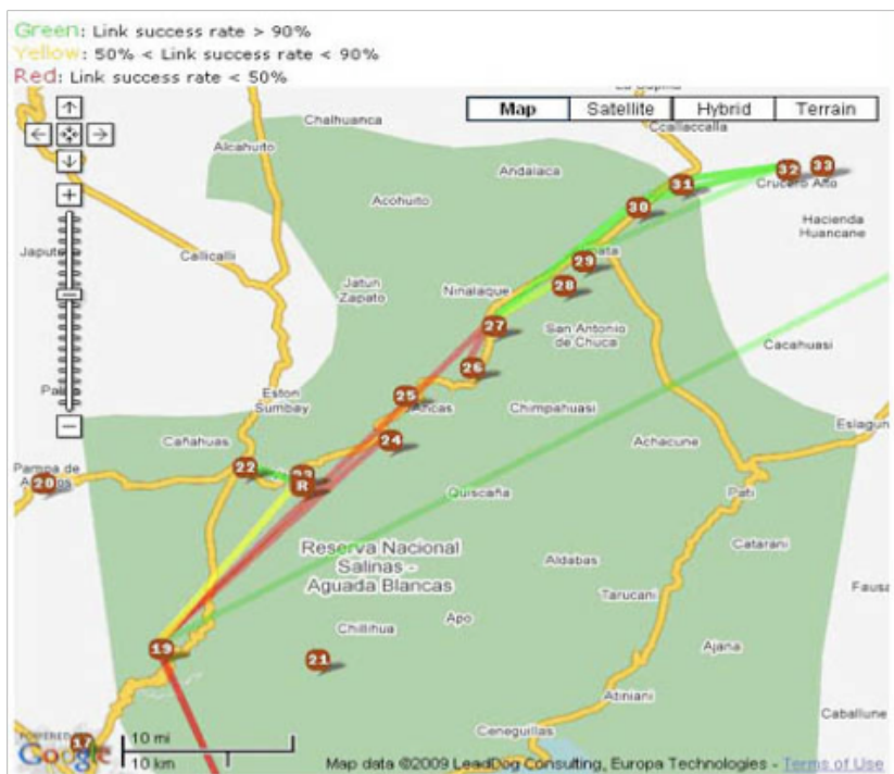
Figure 1: Map of Wireless Link Success in a subsection of the Peru seismic
