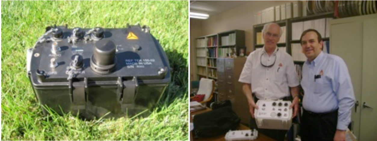
Figure 2. Seismic node for FlexiRAMP Wireless seismic network delivered by Reftek. We propose a 100 station radio-linked network to monitor earthquakes. The digital system and software is of UCLA (Earth and Space Sciences, Civil Engineering, Electrical Engineering, and Computer Sciences) design Reftek president Paul Passmore and engineer Phil Davidson).
