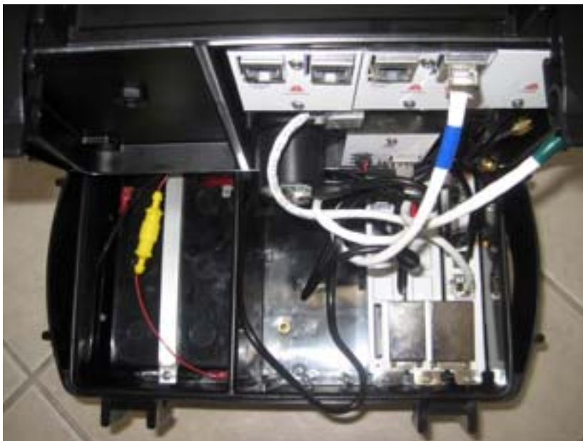
Fig.2. A prototype of the GeoNet box with modular approach inside
