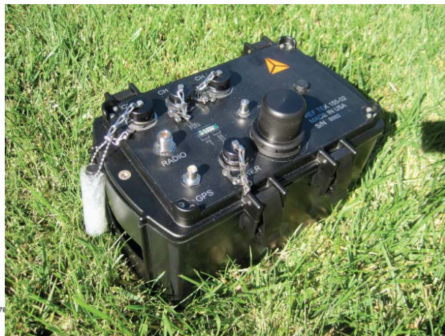
Figure 4. Prototype Reftek EnsBox for GeoNet, SHMnet ShakeNet and FlexiRAMP applications. MEMS seismometer on left. Shielded Circuits include TI A/D, UCLAs LEAP or Crossbow Imote II processor board. Wireless 802.11b card.
