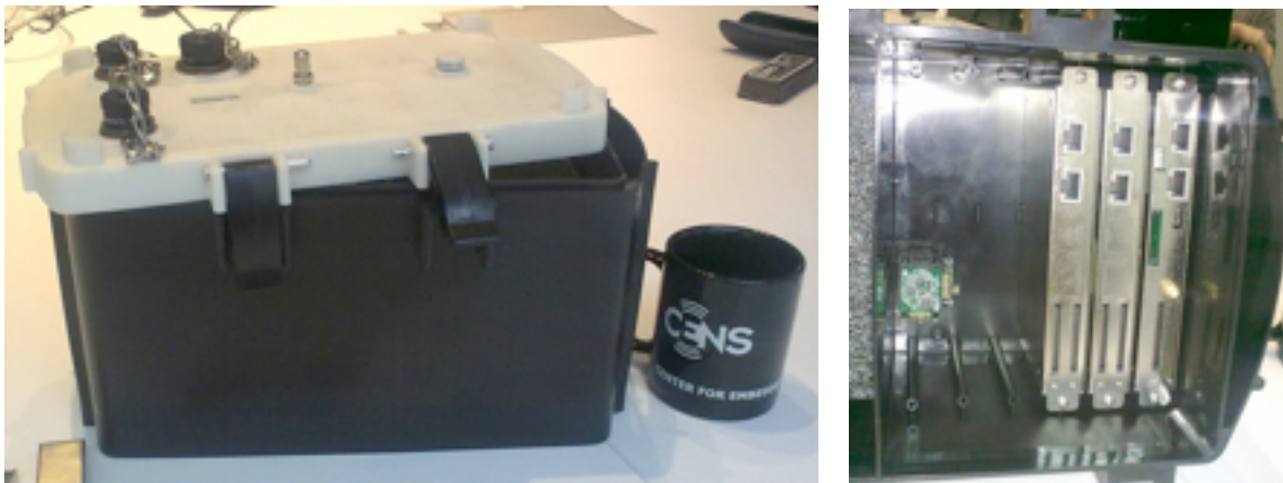
Fig.2. A prototype of a GeoNet box with modular approach inside.
