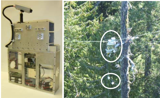
Figure 3. The left-hand image shows a NIMS prototype node system. An imager appears above a package compartment containing embedded computing along with horizontal and vertical actuator components. The right-hand image displays a NIMS node deployed in a forest environment (here at a height of 50m above the forest floor). Suspended from the node is a sensor package that enables sampling of temperature and relative humidity climate variables with solar radiation intensity sensing.
