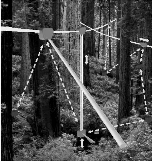
Fig. 2. A schematic view of NIMS, showing mobile nodes suspended on cable infrastructure and its capability for communicating and transporting wireless nodes throughout a three-dimensional volume to provide a network topology adapted to time-varying environmental characteristics.
