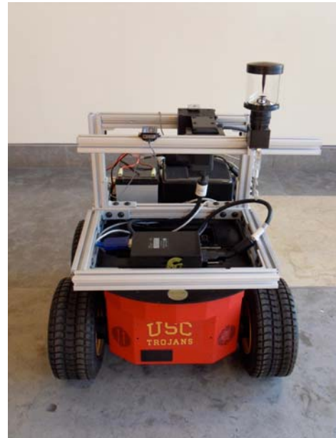
Figure 1. Pioneer 2-AT robot equipped for calibration experiments. The Pioneer carries a NetVision 360 omnidirectional camera and MicroStrain 3DM-GX3 IMU.
