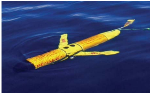
Figure 1: One of our underwater gliders resting at the surface.
