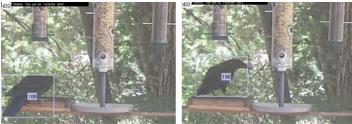
Our approach is able to recognize that detections across with little overlap are the same bird, due to their similar appearance.
