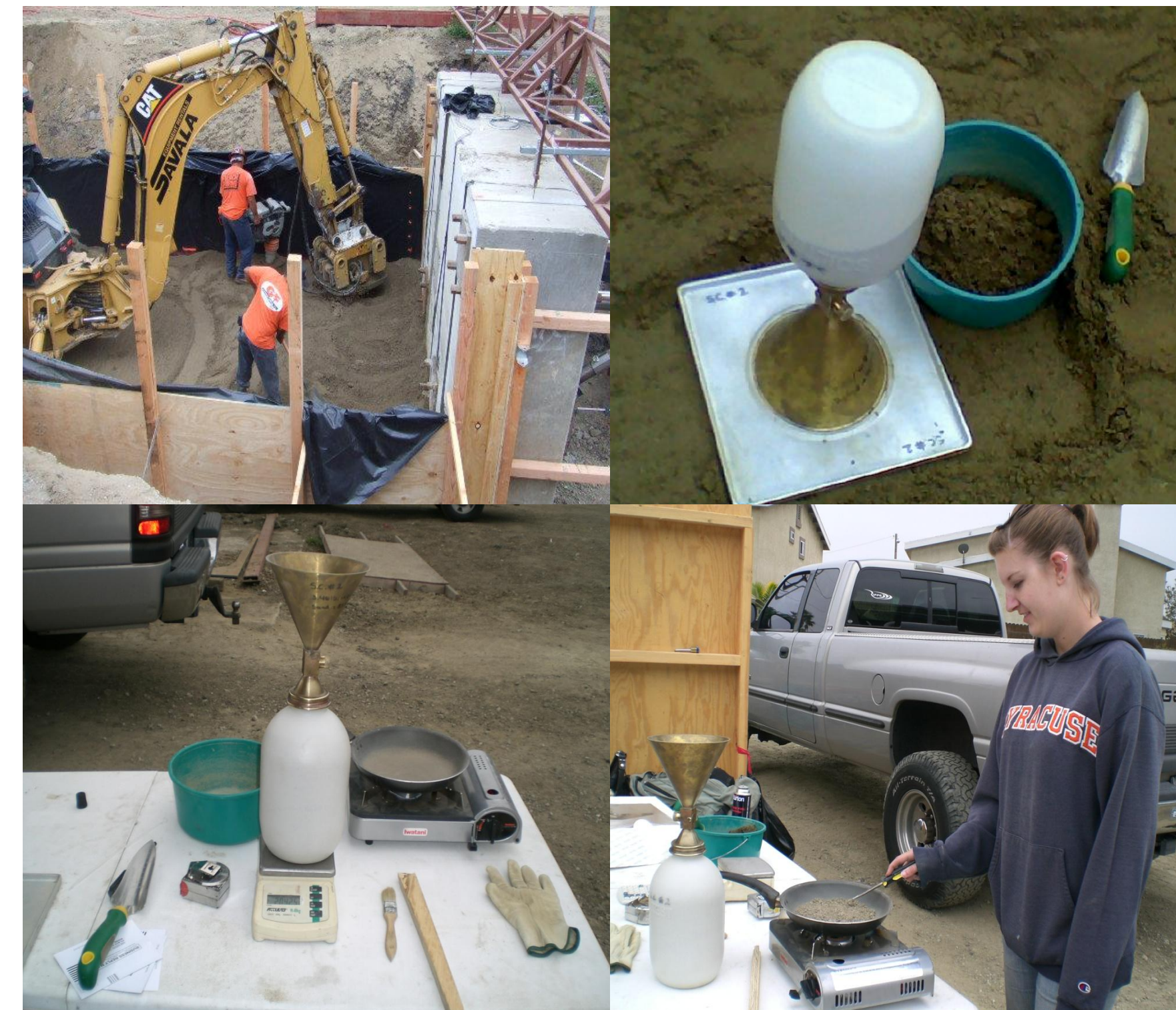
Figure 3: Sand Cone Testing
