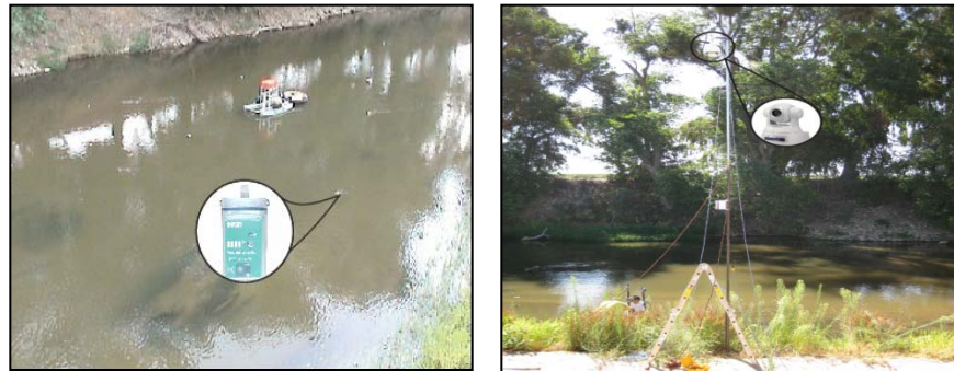
Figure 2 - Light intensity sensors and PTZ security camera used for the river light incidence experiment.
