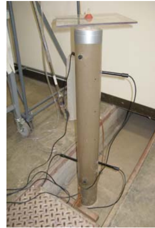
Figure 2. Soil column setup for testing sensor responses under unsaturated soil conditions.
